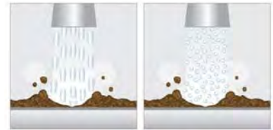
Cold Jet's patented feeder technology creates shaved dry ice on demand.
