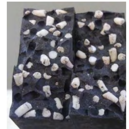
Abrasive grains: resin molding
